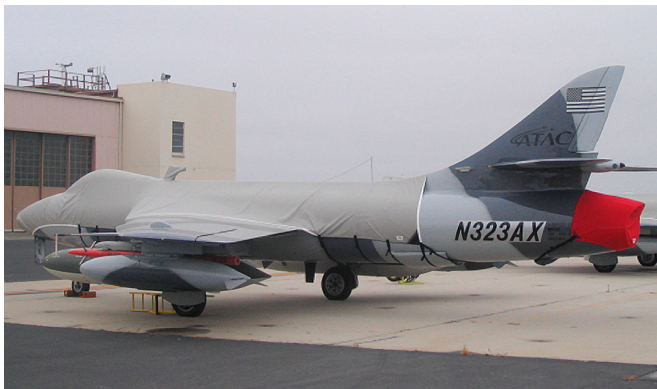
Hunter Fuselage & Exhaust Cover
