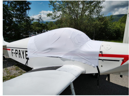
Jodel D113V Canopy Cover, test fit cover
