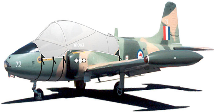
Jet Provost Canopy Cover (Illustration)
