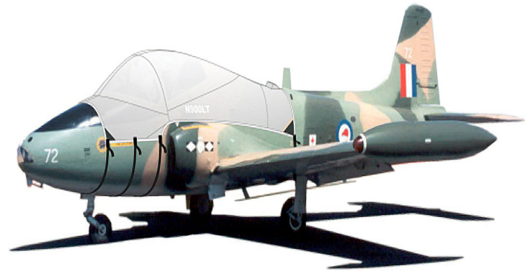
Jet Provost Canopy Cover (Illustration)
