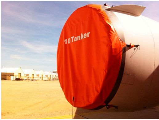
DC-10-30 Intake Cover (CF650C2 Engine)
