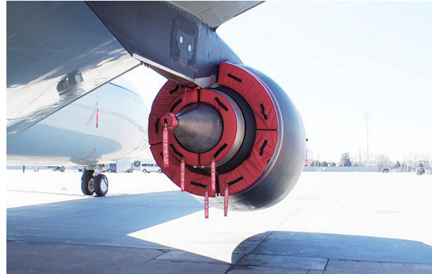
RC-135W Bypass Vent and Exhaust Plugs
