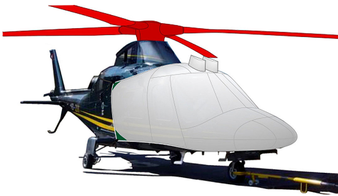
Agusta 109 Bubble, Rotor Hub & Blade Covers (illustration)
