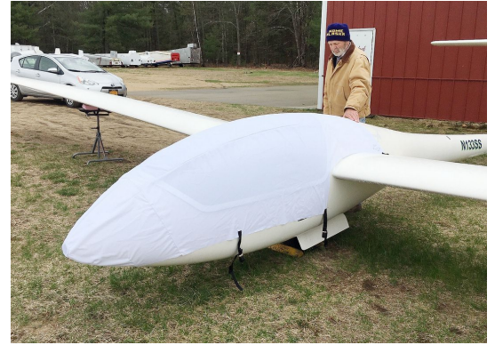
Grob 102 Astir CS Canopy/Nose Cover (test fit)
