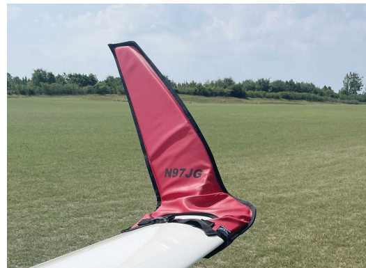
Schempp-Hirth Ventus-2B winglet/wingtip pads
