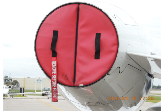
Embraer Legacy 500 Engine Exhaust Plug, folding type
