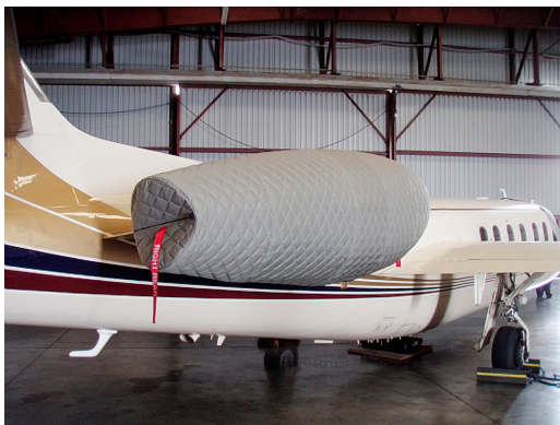
IAI Westwind 1124 Insulated Engine Nacelle Cover
