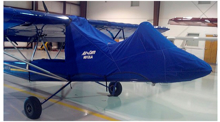
Lockwood AirCam Canopy/Nose Cover w/ aft baggage compartment extension
