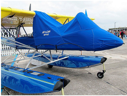
Lockwood AirCam Canopy/Nose Cover w/ aft baggage compartment extension
