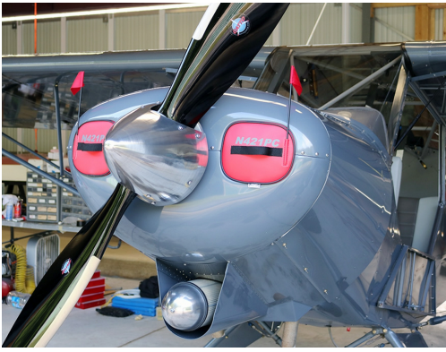
Piper PA-18 Super Cub Engine Inlet Plugs ENGINE PLUGS PREVENT BIRD NEST FOD. Piper Saratoga Engine Cowling Bird's Nest
