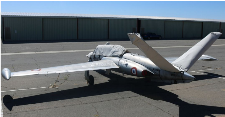
Fougas Magister Canopy/Nose Cover, Tail Stabilizer Covers
