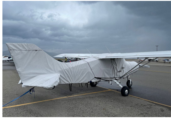
Maule MX7-180 Prop, Engine, Extended Canopy & Empennage Covers
