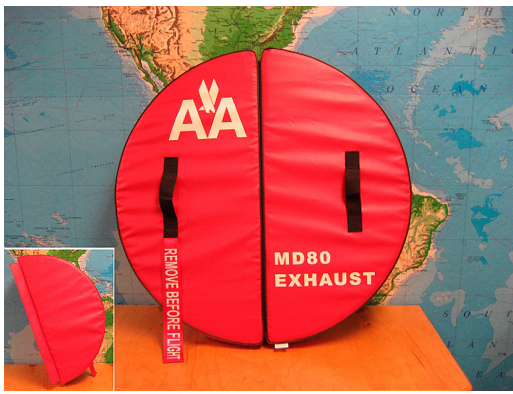
MD-80 Exhaust Plug, folding type
