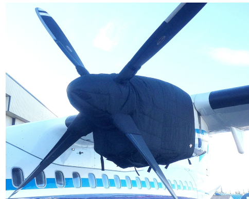
ATR-72-202 Insulated Engine & Prop Hub Covers
