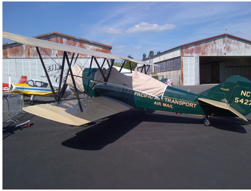
Travelair 4000 Canopy and Engine Cover
