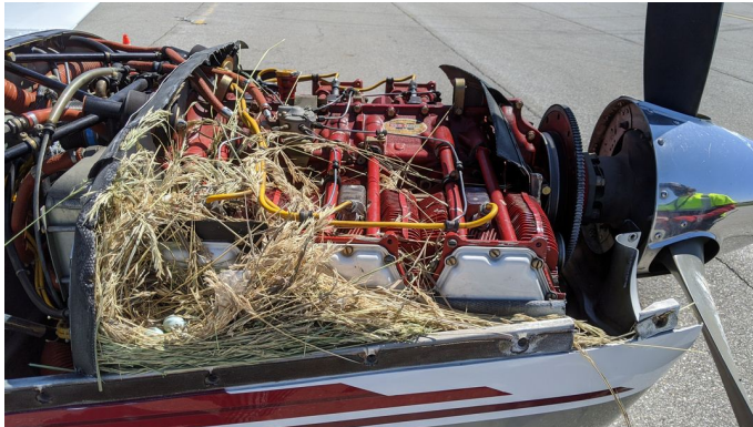
ENGINE PLUGS PREVENT BIRD NEST FOD. Piper Saratoga Engine Cowling Bird's Nest North American TF-51D Exhaust Plugs
