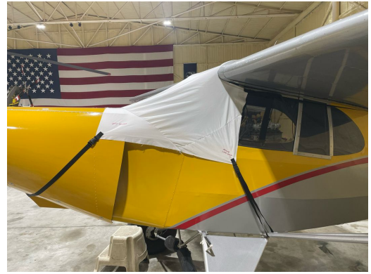
Piper J5A Windshield/Skylight Cover, test fit
