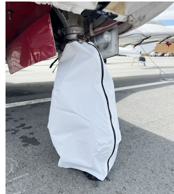
Piper PA-24 Nose Landing Gear Cover, test fit
