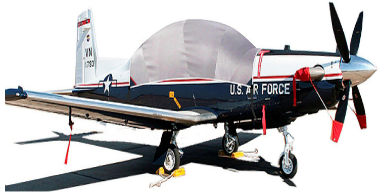
Texan II T6A Canopy Cover, Engine Inlet Plug, Prop Tie/Exhaust Covers, Pitot Cover
