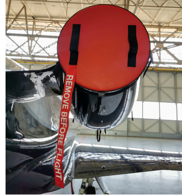
Embraer Phenom 300 ENGINE INLET COVERS & EXHAUST PLUGS (includes lower nacelle plug) (set of 6)
