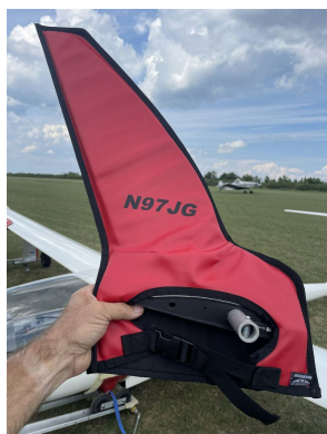
Schempp-Hirth Ventus-2B winglet/wingtip pads
