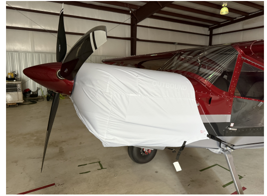
Rans S-21 Engine Cover, test fit cover
