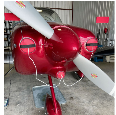
RV-14A Engine Inlet Plugs, Sam James Cowl
