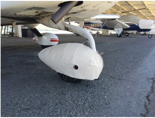
Grumman AA5 Nose Wheelpant Cover, test fit
