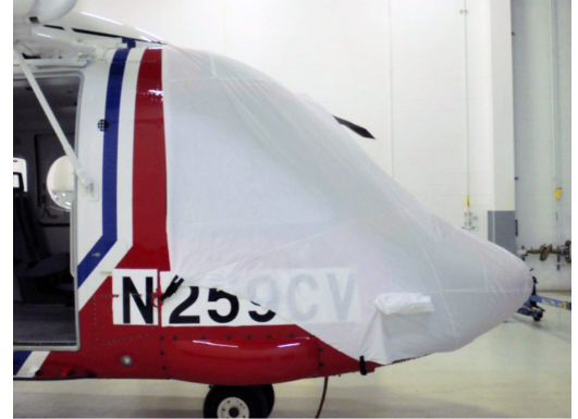
Sikorsky S-92 Windshield/Nose Cover, test fit cover
