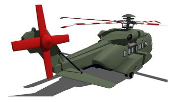
Sikorsky S-92 Main Rotor Mast Cover, Insulated, w/Heater Hose Inlets
