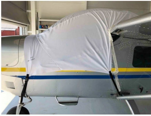
Saab Safari Canopy Cover, test fit cover
