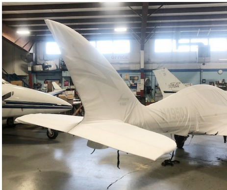
Shark 600 Complete Cover Set, test fit
