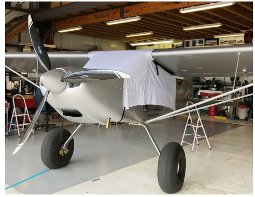
Rans S-20 Canopy Cover, test fit cover
