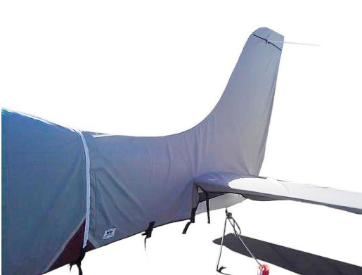
Cirrus SR20 Empennage Cover (covers tail boom, vertical and horizontal stabilizers)
