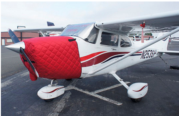
Cessna 172 Insulated Engine Cover, fully enclosed
