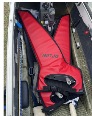
Schempp-Hirth Ventus-2B winglet/wingtip pads
