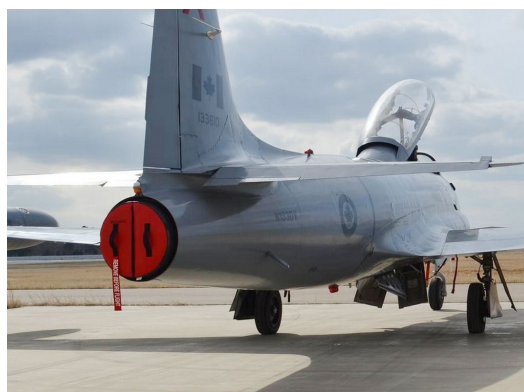
Lockheed T-33 Shooting Star Exhaust Plug, Folding Type
