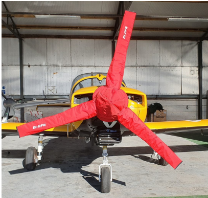
Slingsby T-67 Firefly Insulated Propellor/Spinner Cover
