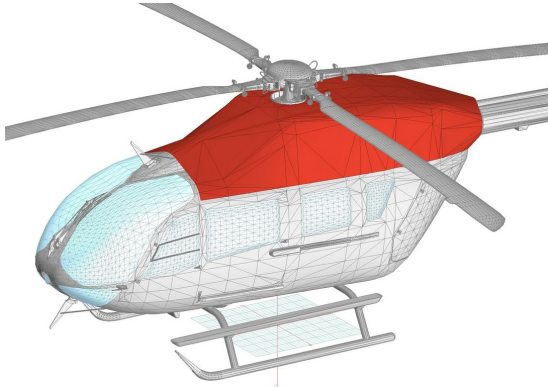
Intake/Exhaust Engine Area Cover, 3D Rendering
