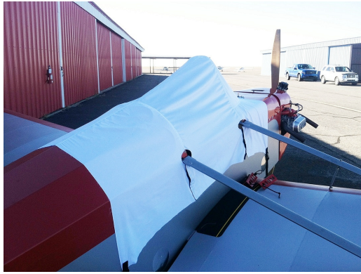
Volksplane Canopy Cover (test fit cover)
