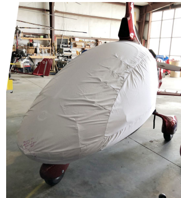
Cavalon Gyrocopter Bubble Cover, test fit cover
